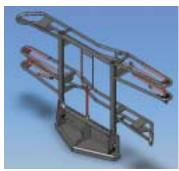
An innovative business partnership between Midwest Bus Corp. and Altair Engineering has resulted in the successful launch of bike racks for buses. When deployed (left), the rack protrudes less than 36 in. from the front bumper; when stowed (right), it protrudes less than 7 in.
