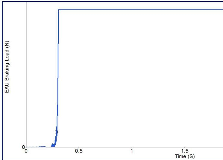
**Figure 5: Braking load curve for FE model of EAU**
