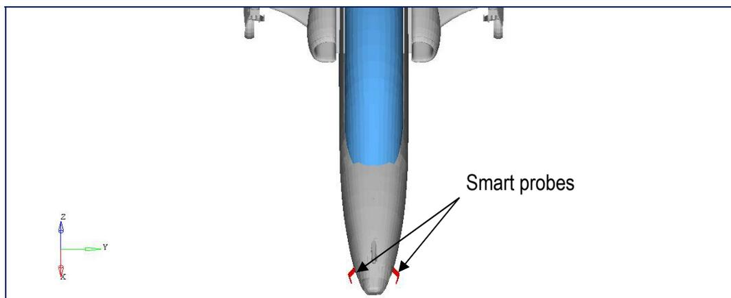
**Figure 2: Location of Smart Probes on Nose of Aircraft**
