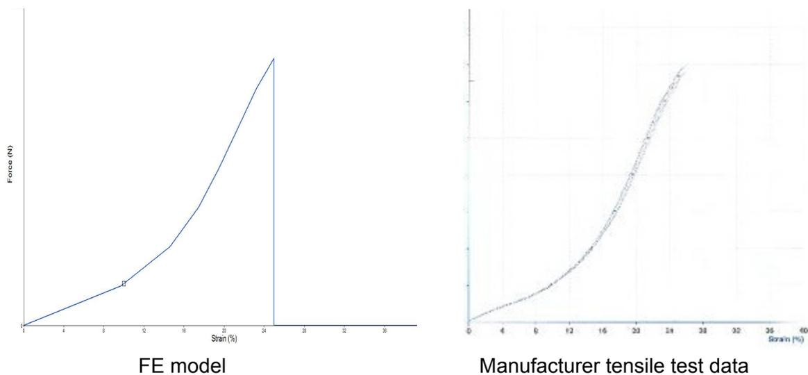
**Figure 4: Correlation of Force/Extension behaviour for Main Net Webbing**
