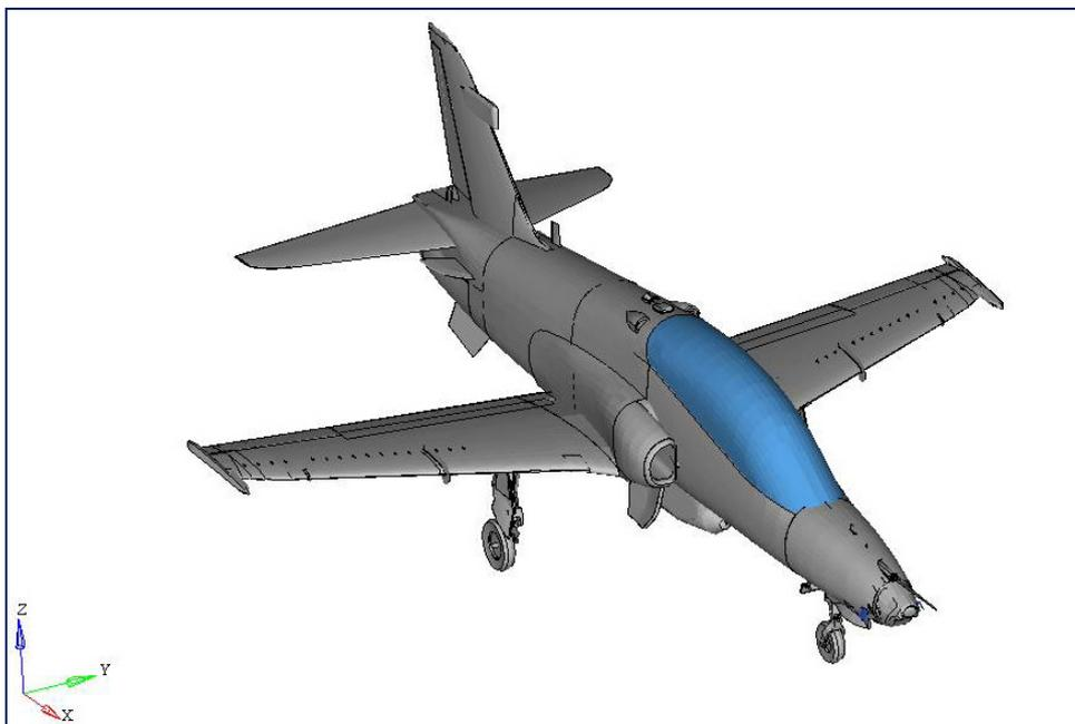
**Figure 1: RADIOSS FE Model of Hawk T Mk2 Aircraft**
