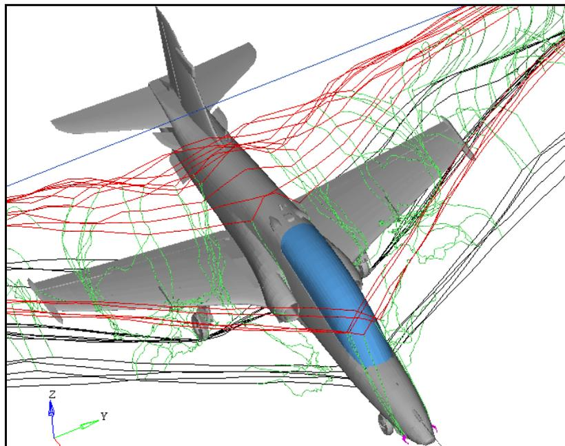
**Figure 9: Separation of Barrier Nets from Central Support Cable**
