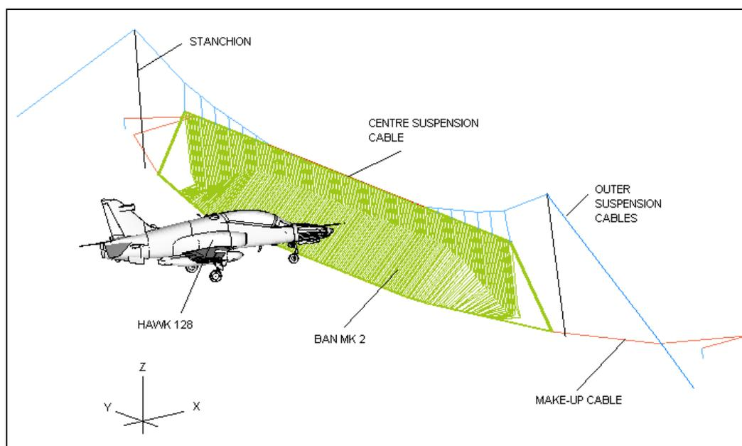
**Figure 3: Layout of Barrier Net Model**
