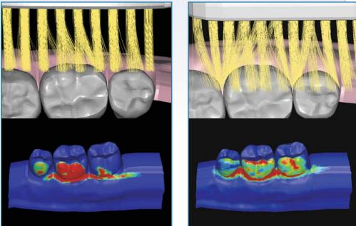
Altair engineers helped Lion use RADIOSS to set up the odonto-gnathic simulation. Engineers also analyzed the loads and displacements on the handles, whose functions are to absorb stress and minimize pressure on the teeth and gums. Then, engineers analyzed the contact friction energy of both brushes' bristles to the teeth, comparing the same range of motion after two reciprocating movements.
