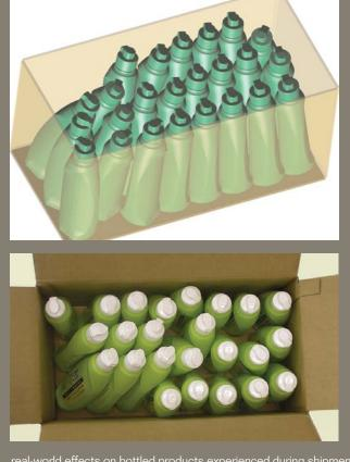
real-world effects on bottled products experienced during shipment and consumer use. The goal of these simulations is to minimize the amount of material used and to prevent product leakage when the
