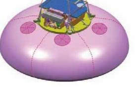
ing to rest, takes typically less than 100 milliseconds and results in decelerations of up to 80g.
