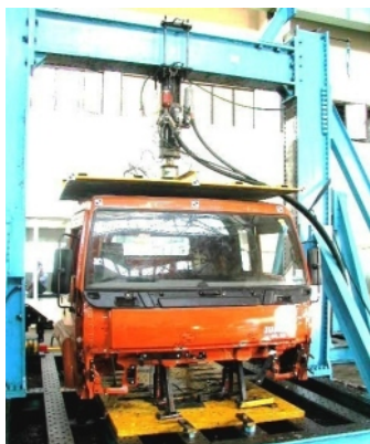
Figure 4 Physical test setup
