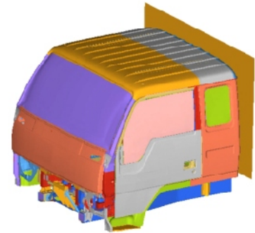
Figure 2 Numerical simulation of rear wall strength test
