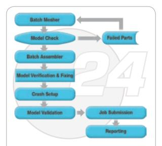
The Altair team completed a full frontal vehicle crash analysis – which typically takes weeks – in just 24 hours using only commerically released software in Altair HyperWorks. and managed with Altair's embedded simulation data management solution.
