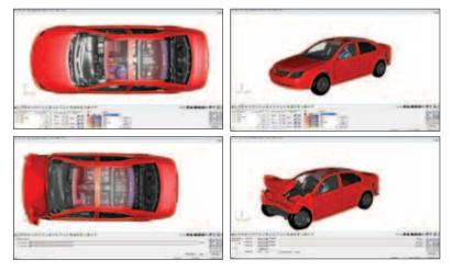
For the CAD2CRASH24 proof-of-concept, Ford supplied the BIW CAD model while the subsystem models from the National Highway Traffic Safety Administration were morphed to fit the BIW model. The top images (from left to right), show the top and iso views of the vehicle prior to the crash while the bottom images (left to right) show the crash results using Altair HyperView.
